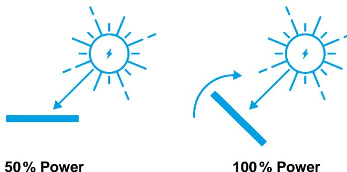
By opening the FLIN clamp, the system can be aligned to the sun via the adjustment lines in order to exploit the full power. To do this, push the buttons of the clamps (in the corners of the module) and pull the solar module in order to align it with the sun and the sun's rays ideally fall
